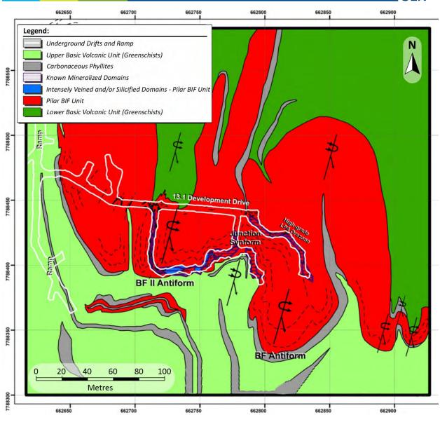
Figure 7-7: Schematic Geological Setting - Level 13.1, Pilar Mine
