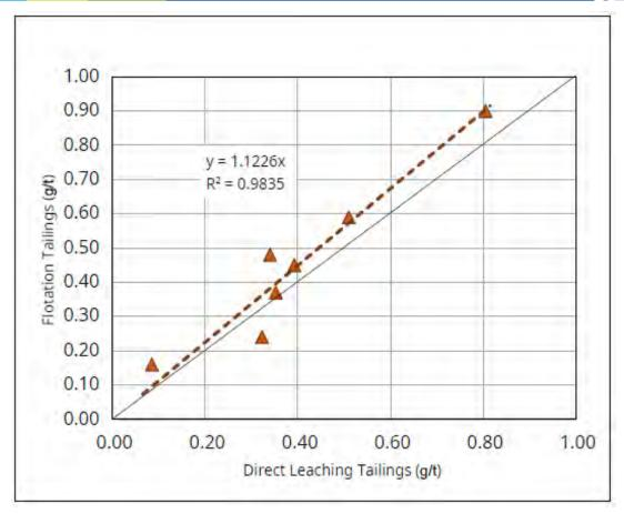
Figure 13-15: Flotation/CIP Tailing Assay Correlation
