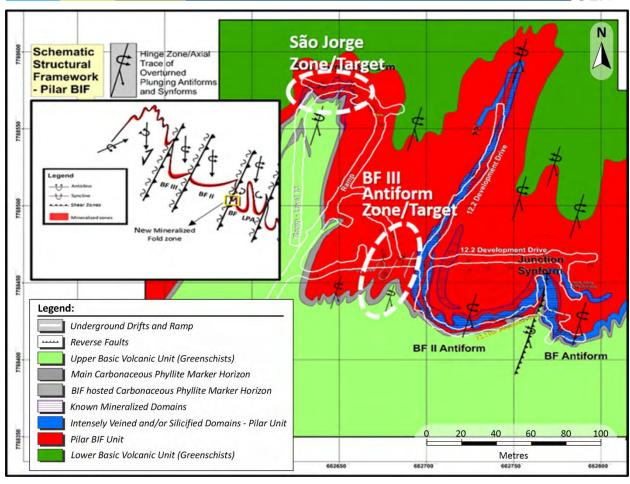
Figure 7-18: Schematic Geological Setting Level 12.2. "Composite" with Zones/Targets,
