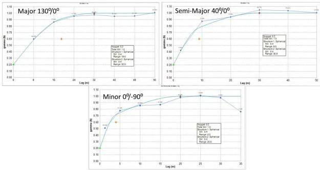
Figure 14-48: Correlogram for Oxide Mineralization
