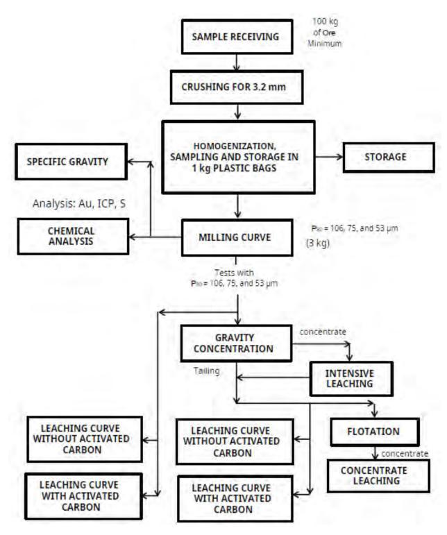
Figure 13-1: Metallurgical Test Work Flowsheet
