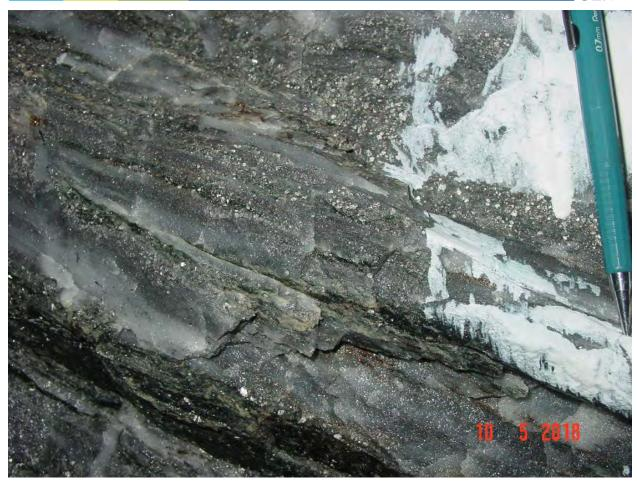
Figure 7-24: Typical "Sulphide-Facies", High Grade, Arsenopyrite-Rich BIFs at Pilar Sublevel 10.2
