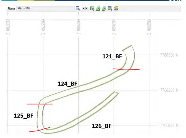
Figure 14-31: Example of Wireframe Sub-Boundaries for Soft Domain Estimation, Pilar Mine
