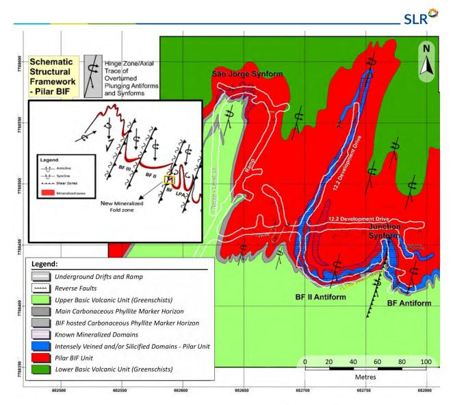
Figure 7-6: Schematic Geological Setting - Level 12.2 "Composite", Pilar Mine
