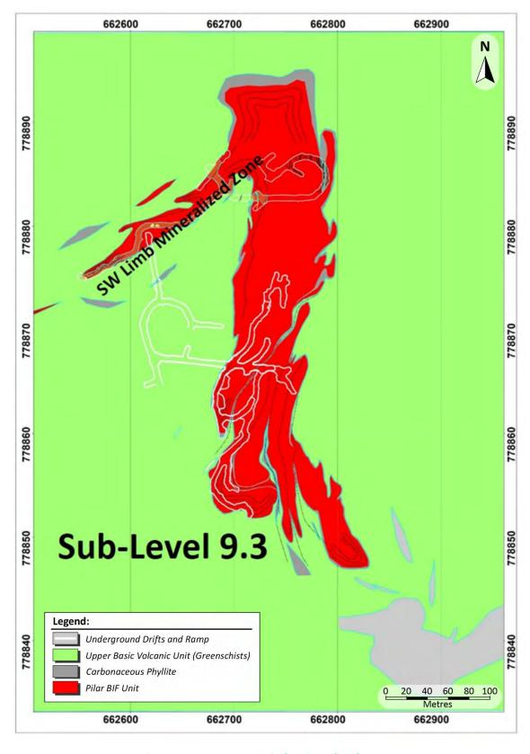
Figure 7-20: SW Limb Mineralized Zone
