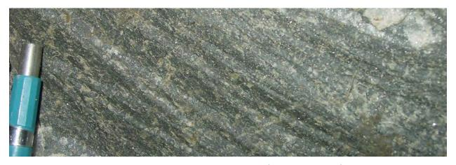
Figure 7-9: Main Penetrative Tectonic Cleavage (Main Schistosity), Pilar Mine
