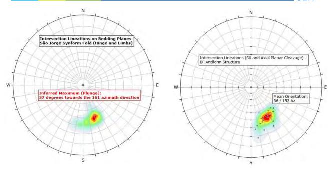
Figure 7-13: Distribution of Attitudes of Main Penetrative Intersection Lineation in São Jorge Synform, Level 12 (Left) and BF Antiform, Level 10 (Right)
