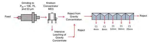
Figure 13-2: Flotation Test Scheme
