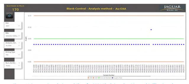
Figure 11-2: Sample Control Chart for 2021 Blank Samples, Diamond Drilling Samples
