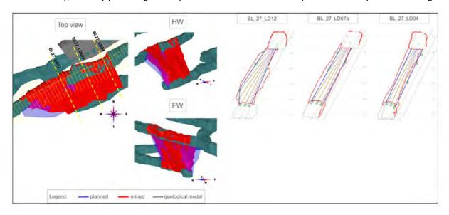
Figure 16-2: Typical Stope Layout
