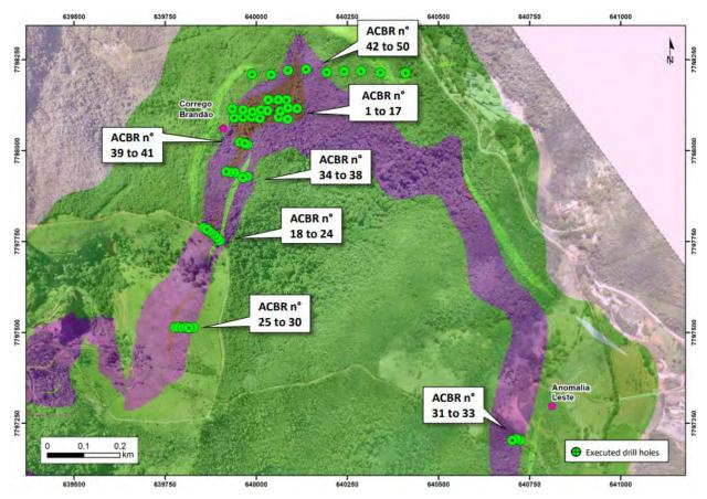
Figure 10-3: Auger Drill Holes, Córrego Brandão Deposit and Anomalia Leste Target
