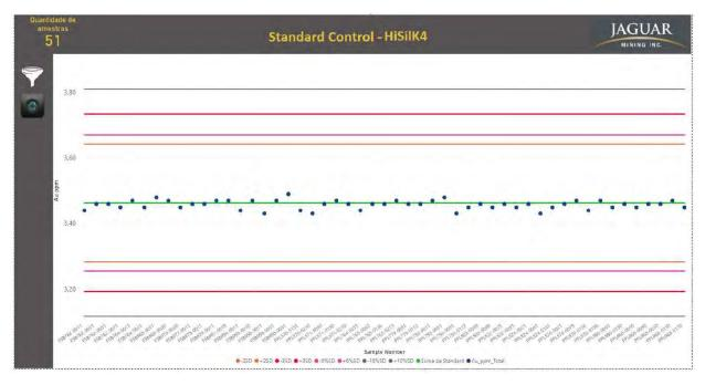
Figure 11-4: Sample Control Chart for Standard Reference HISILK4, 2021 Diamond Drill Hole Samples
