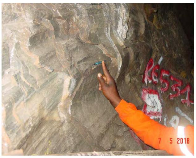
Figure 7-12: Typical Penetrative Intersection Lineation on Folded Bedding (S0) Surfaces of the Pilar BIF Unit (Level 10)
