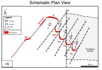
Schematic map showing the main structures in the Pilar mine. The Torre block that hosts the Torre mineralization is thrust over the Pilar domain.
