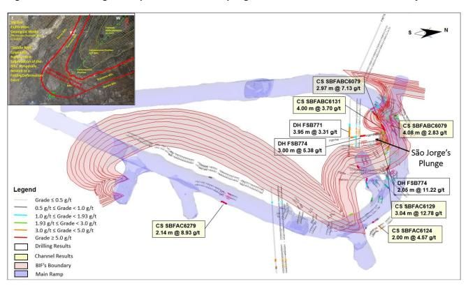
Figure 4. Plan showing development channel sampling, diamond drill hole location and assay results.
