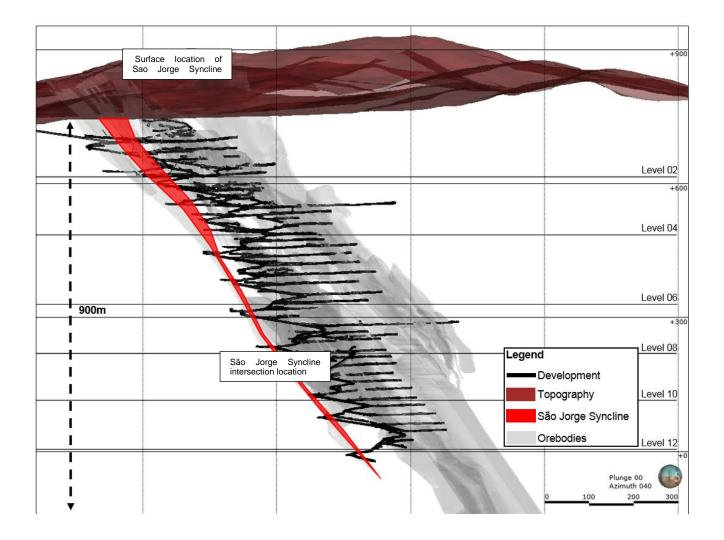
Figure 3. Plan View showing the location of the Sao Jorge Syncline at Pilar Mine relative to the SW trend, the BF2, BF and BA orebodies and current mine operational areas on levels 12- 13.
