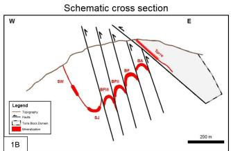
Schematic cross section showing the main structures in the Pilar mine and the BA, BF, and BF2 sequence of BIF hosted orebodies within antiforms. At Torre mineralization is associated will fine grained arsenopyrite disseminated with sericite-quartz
