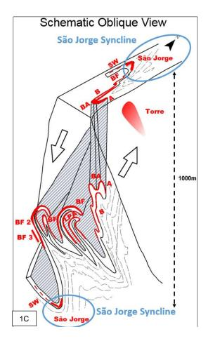
Figure 2. Pilar Long Section showing location of Sao Jorge Syncline at surface and close to 13 level where it was intersected by development relative to the BIF Orebodies (BF2, BF, and BA).
