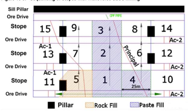
Figure 16-3: Sequencing of Stopes with Transverse SLOS Mining
