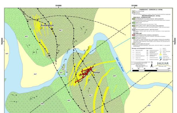
Figure 9-1: Pontal Deposits Geology Map Showing Underground Drift and Ramp
