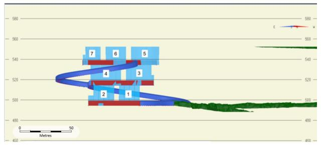
Figure 16-5: Typical Drilling Layout with Longitudinal SLOS
