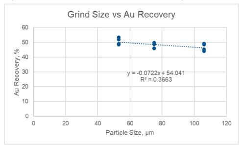
Figure 13-8: SF1 Grind Particle Size vs Au Recovery
