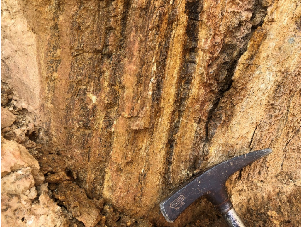
Figure 7-9: Moderate to High Grade Veined Amphibolite at the Bottom of the Faina Open Pit
